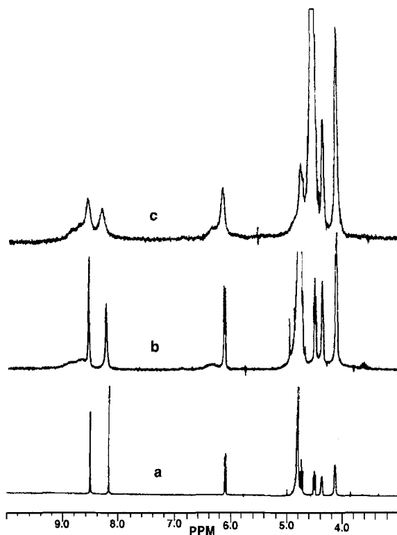
FIGURE 1 1 H NMR spectra of (a) AMP at 20°C, (b) AMP:RTD = 3:1 at 20°C, (c) AMP:RTD = 3:1 at 45° C in D 2 O/CD 3 COCD 3 = 9/2 using DSS as standard.
